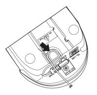
4. Plug one end of the long telephone cord into the **TEL LINE** jack on the Base Unit.
